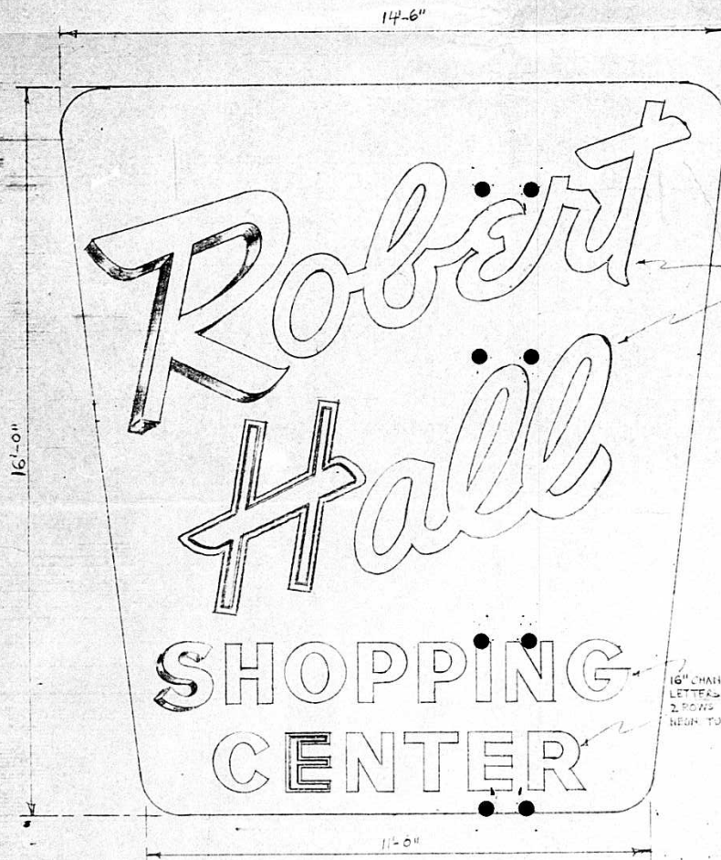
FACE VIEW OF DOUBLE FACE ILLUMINATED PYLON SIGN SCALE \frac{1}{4}"=1'-0"
