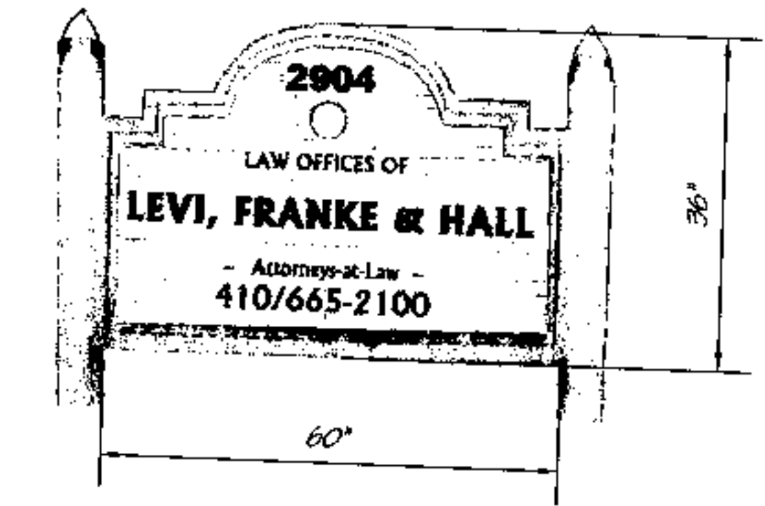
DETAIL: FREESTANDING I.D. SIGN SCALE: 1/8"=1'-0"
