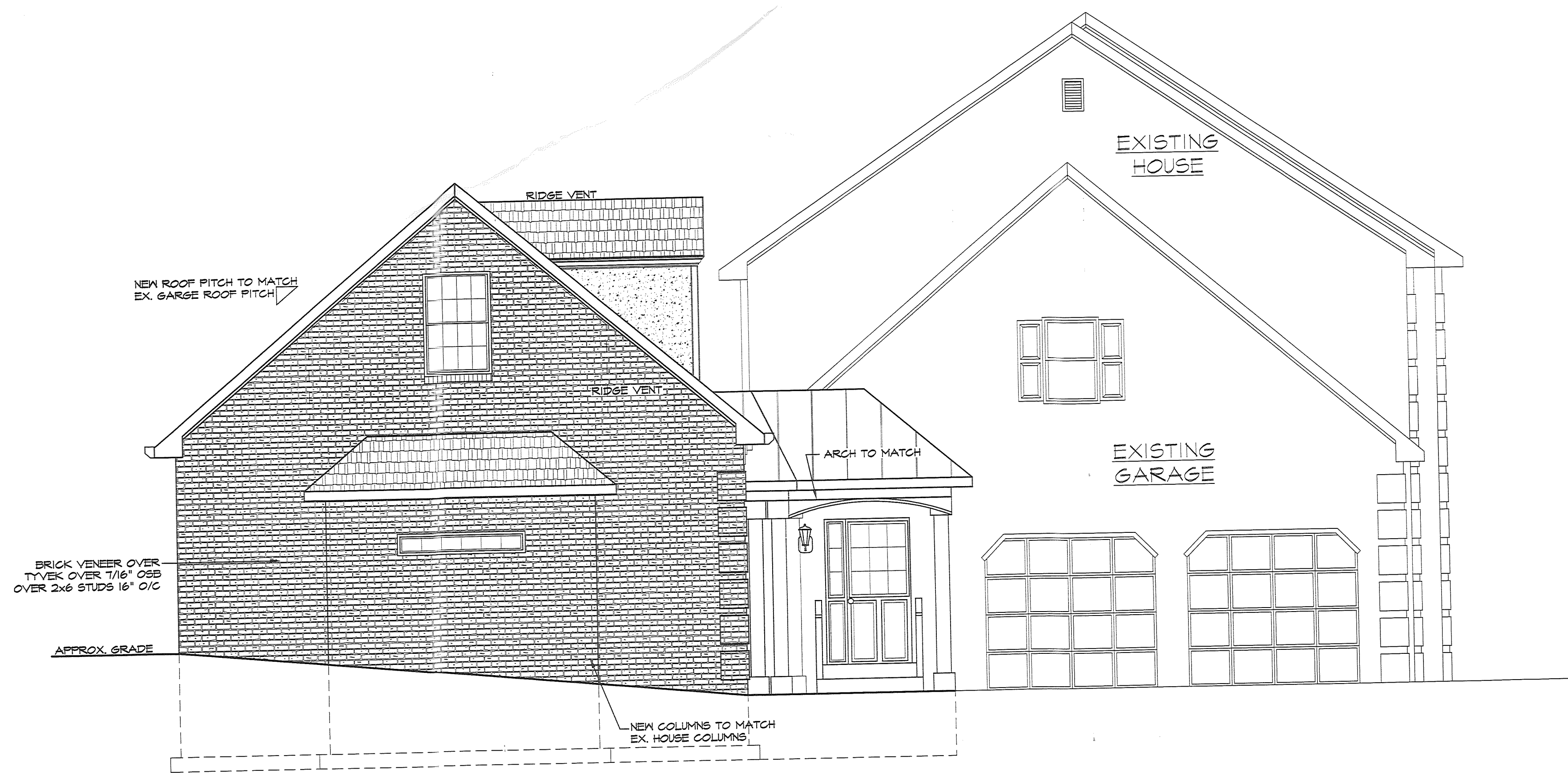
LEFT SIDE ELEVATION SCALE: 1/4"=1'-0"
