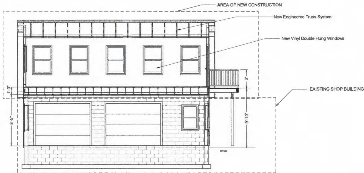
CROSS SECTION FRONT VIEW SCALE - 1/4" = 1'0"
