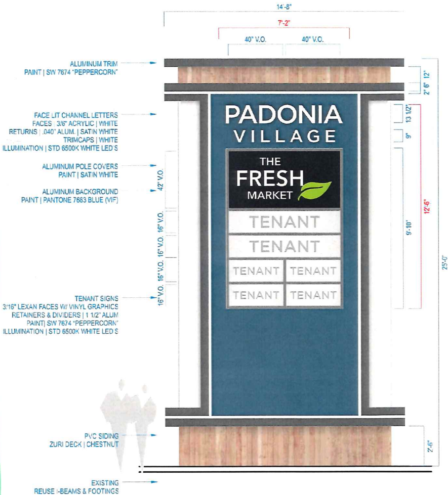
SIGN C PROPOSED PYLON SIGN | ELEVATION Scale: NTS QTY. REQ'D: ONE (1) 89.6 sq. ft.
