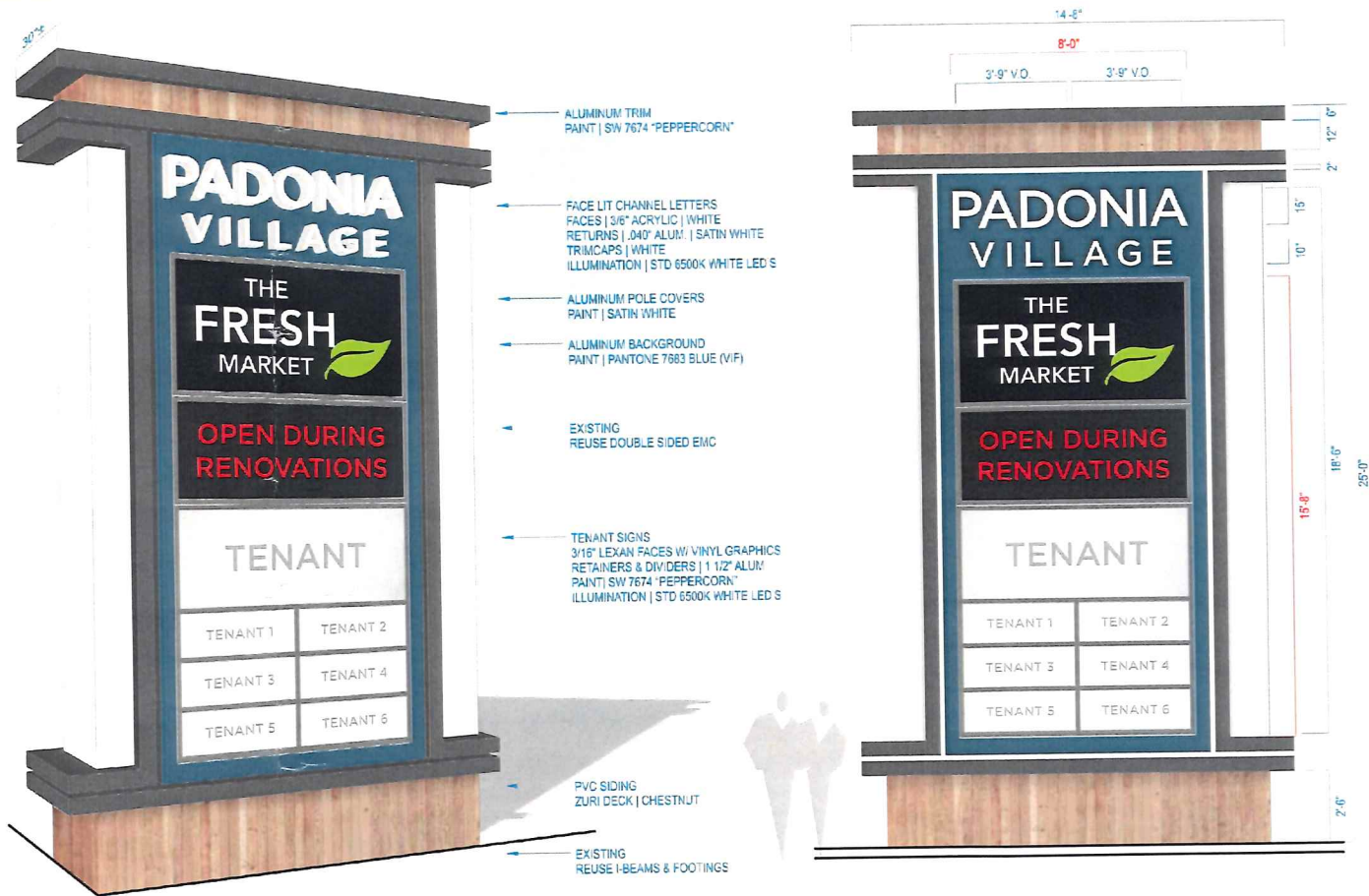
SIGN B PROPOSED PYLON SIGN | ELEVATION Scale: NTS QTY. REQ'D: ONE (1) 148 sq.ft.
