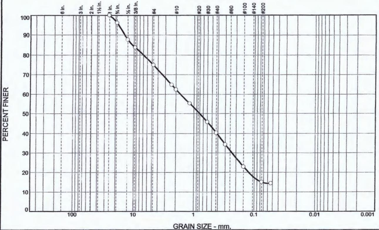
ASTM Specifications performed may include: D421, D422, D2216, D2217, and D4318.
