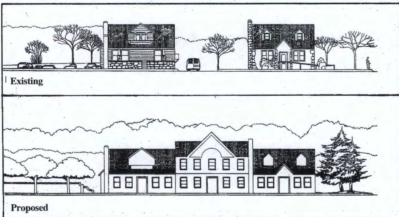
An example of adaptive reuse -- two existing residences were remodeled, and linked with an addition, to become a compatible, leasable commercial building.
