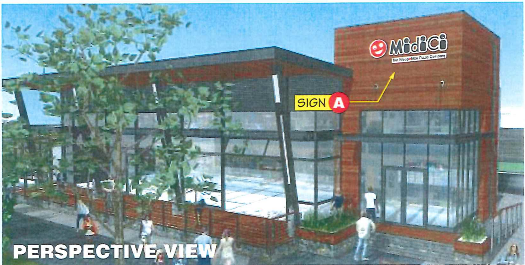
EL-1 FRONT/ EXTERIOR ELEVATION - MP-2.5A-CBG QTY: (1) 1'-6 1/2" CHANNEL LETTER SIZE SCALE: 1/4" = 1'-0"
