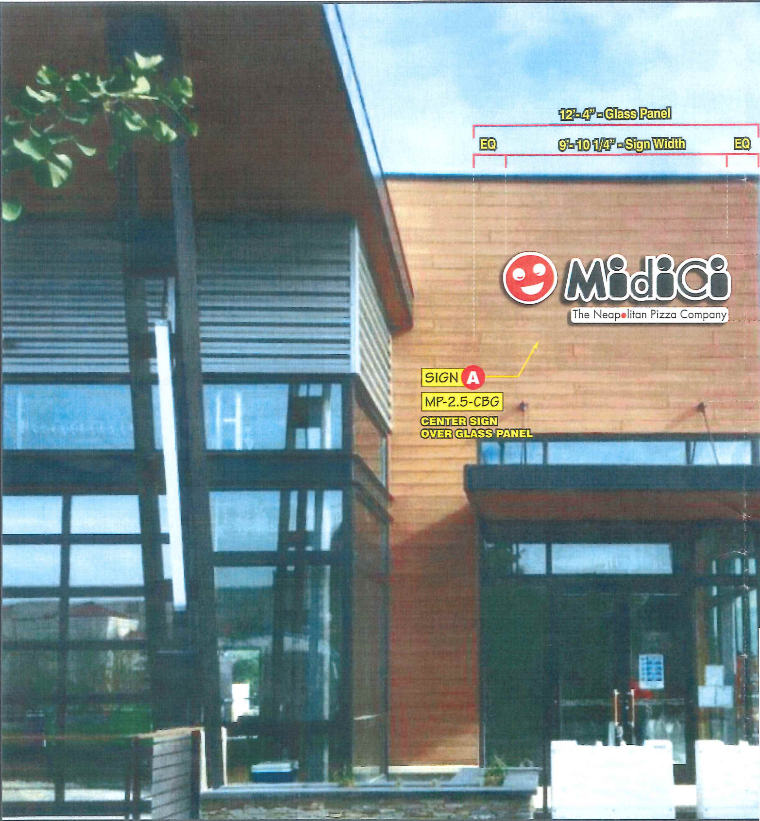
EL-1 FRONT/ EXTERIOR ELEVATION - MP-2.5A-CBG QTY: (1) 1'-6 1/2" CHANNEL LETTER SIZE SCALE: 1/4" = 1'-0"
