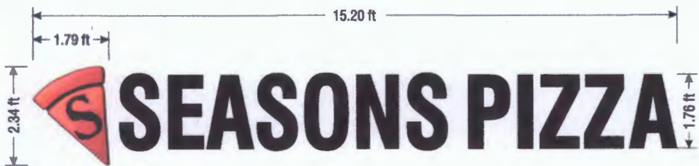
SIGN TYPE: A (Qty:1) Left Elevation LED Illuminated Channel Letters & Logo (Remote Mount) (35.56 Square Feet)
