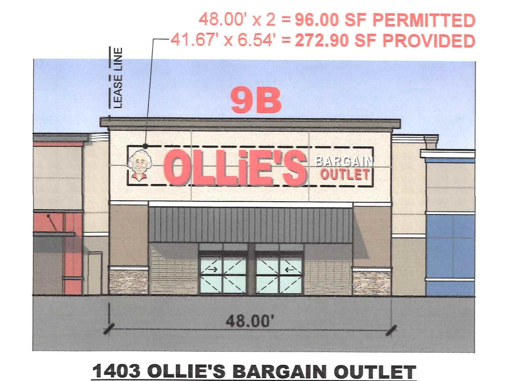
ELEVATION "F" (45 DEGREES TO MERRITT BLVD.)
