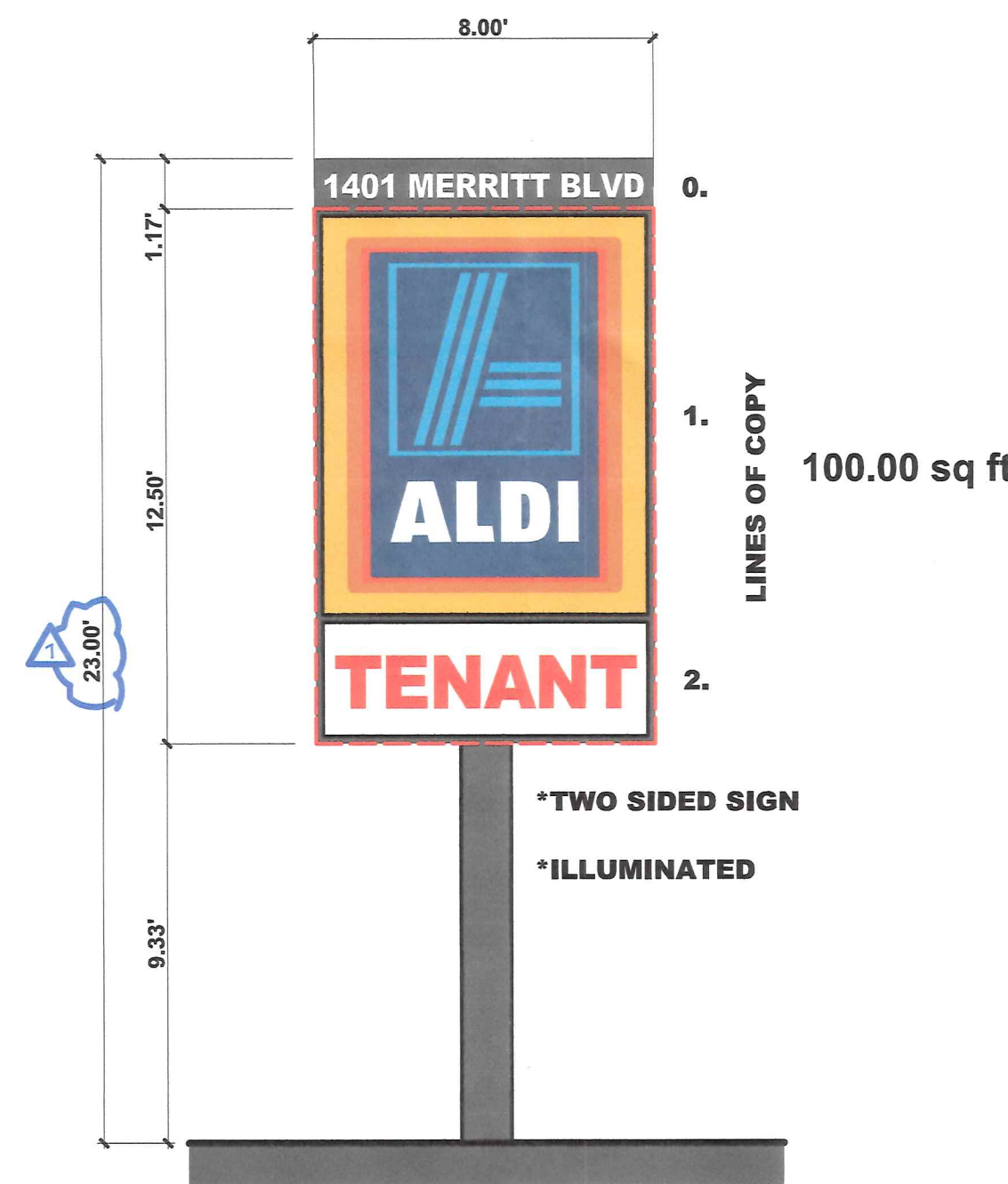
C. PROPOSED FREESTANDING JOINT IDENTIFICATION SIGN MERRITT BLVD ENTRANCE SCALE: 1/4" = 1'-0" SIGN AREA: 8.00' x 12.50' = 100.00 ft 2 (NOT INCLUDING PROPERTY IDENTIFICATION AND COLUMN) LETTER HEIGHT: HEIGHT OF COPY MAY BE LESS THAN 8", BUT ALL MUST BE GREATER THAN 3"
