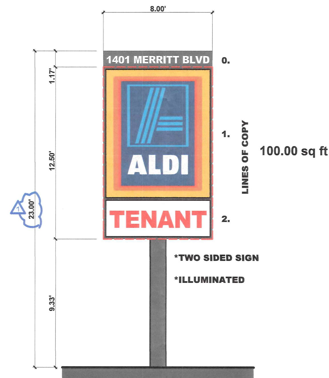
C. PROPOSED FREESTANDING JOINT IDENTIFICATION SIGN MERRITT BLVD ENTRANCE SCALE: 1/4" = 1'-0" SIGN AREA: 8.00' x 12.50' = 100.00 ft 2 (NOT INCLUDING PROPERTY IDENTIFICATION AND COLUMN) HEIGHT OF COPY MAY BE LESS THAN 8", BUT ALL MUST BE GREATER THAN 3" LETTER HEIGHT:
