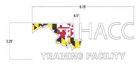
1.5" DEEP, FABRICATED STAINLESS STEEL REVERSE CHANNEL LETTERS, PAINTED WHITE (FACE & RETURNS) INTERNALLY ILLUMINATED WITH HALO EFFECT LED
