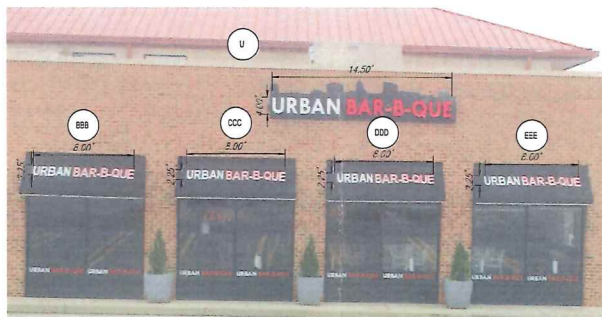
BUILDING 1 WEST ELEVATION NOT TO SCALE BLD1WB
