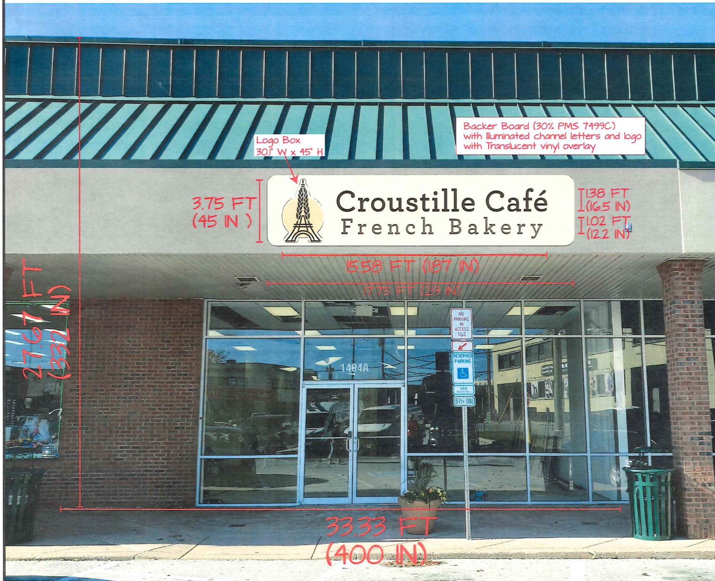
Illuminated Channel Letters on Backer Board
