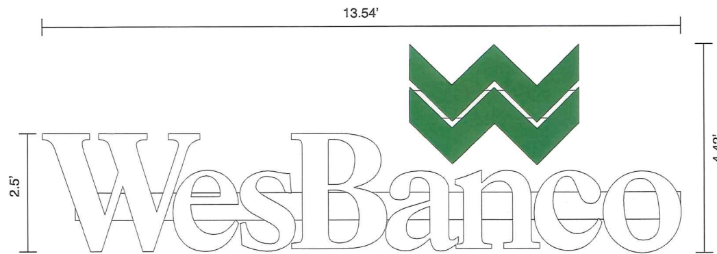
Face-lit channel letters on raceway
