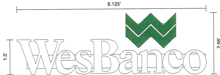
Face-lit channel letters on raceway
