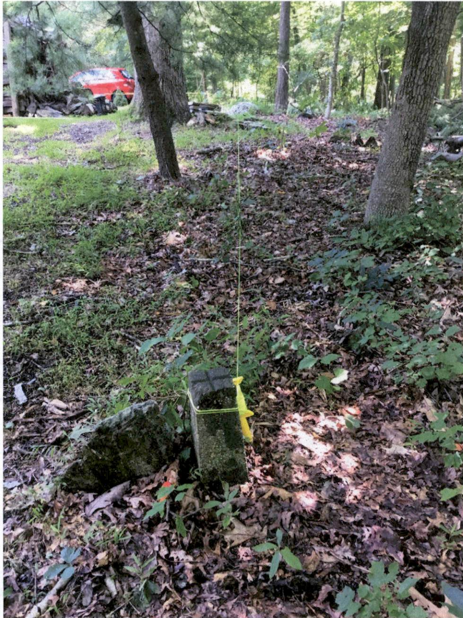
Photo 4: This photo shows concrete monument No. 76 as described in the property Deed and is the POB of the property line stake out. The photo is looking South 51 degrees 8 minutes and 32 seconds ( S 51 08' 32" E) as described in the property deed. The yellow line has been placed between concrete monument No. 76 and the stake placed adjacent to Spooks Hill Rd. (2 nd POC as described above) at a distance of 236 feet.
