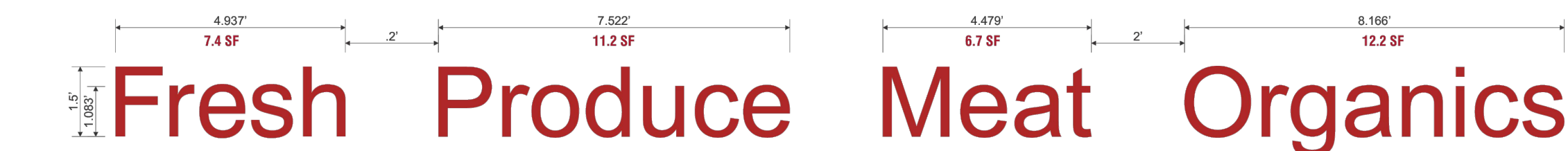
2 18" LETTER HEIGHT : FACE-LIT REMOTE CHANNEL LETTERS (1) ONE SET REQUIRED
