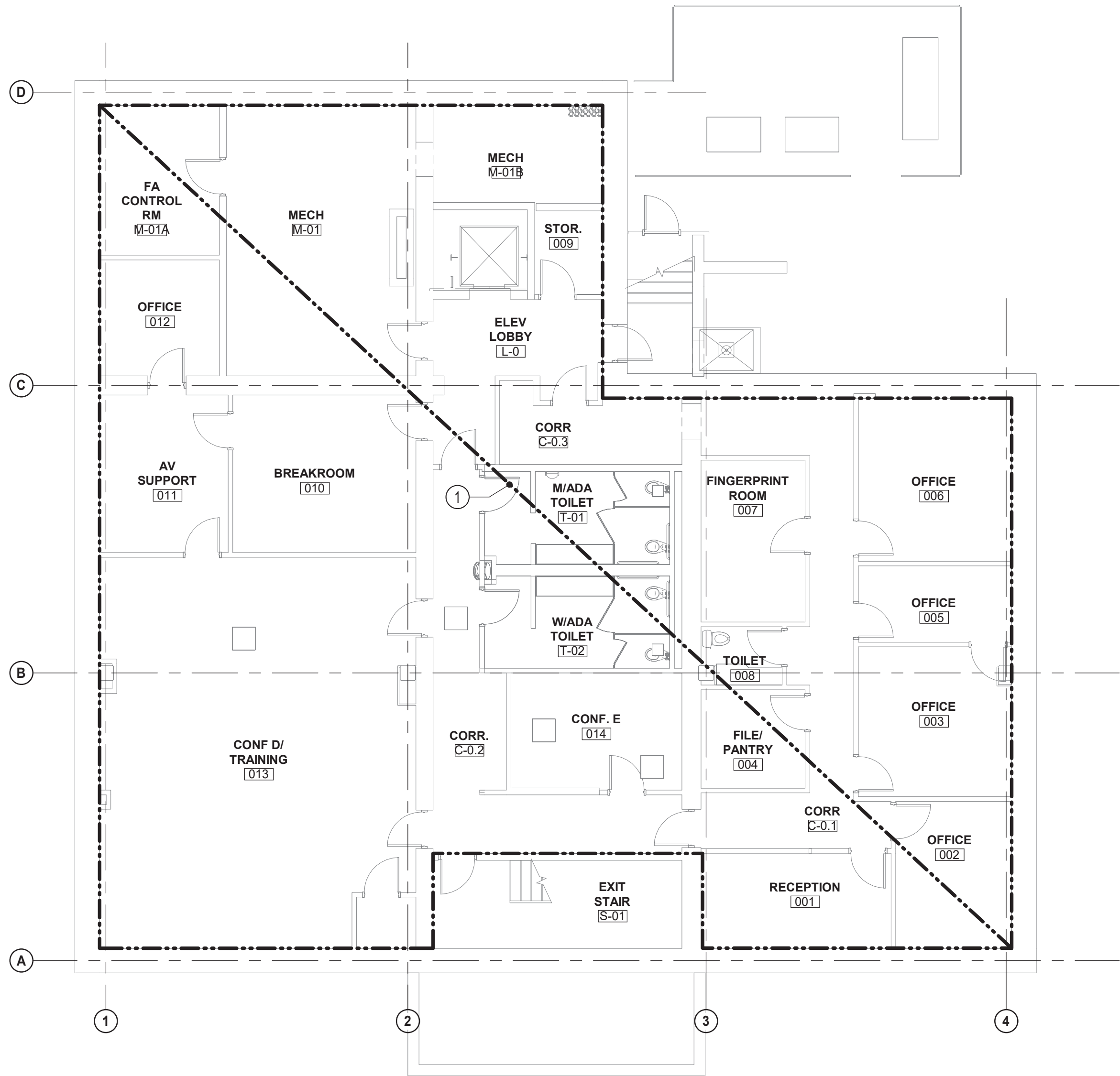
1 GROUND FLOOR PLAN - FIRE PROTECTION - NEW WORK 1/8" = 1'-0"
